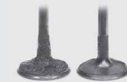
Intake Valve before P.I. Treatment
