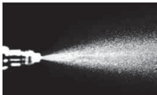
Injector spray pattern after P.i. treatment.
